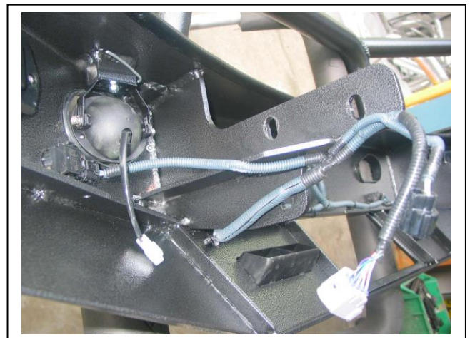
Figure 12: Secure wiring in rear of channel. NOTE wiring direction secured to mount.
