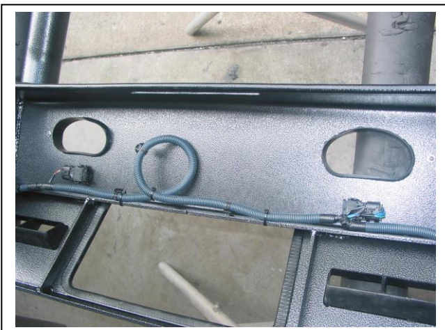
Figure 11: Secure wiring in rear of channel. Parking sensor wiring shown.
