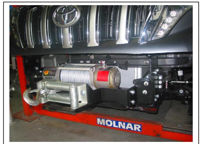
Figure 6: ECB Winch frame with test winch fitted
